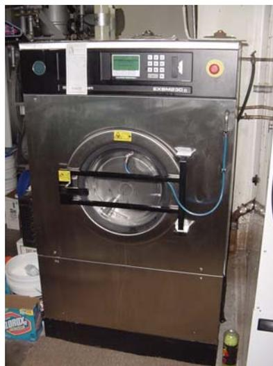
Computerized washer used in the wet cleaning process.
