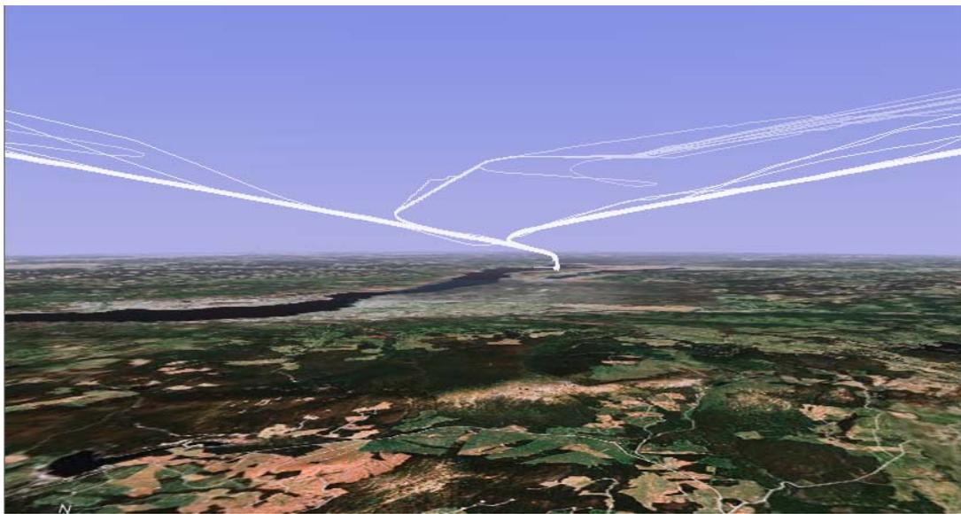
*Side view of the same approach paths after the RNP Approach System is implemented. The same results can be achieved in New York with a resulting flow of single lines replacing the many different lines shown in Figure 19. (Source: Naverus Corp.)*
