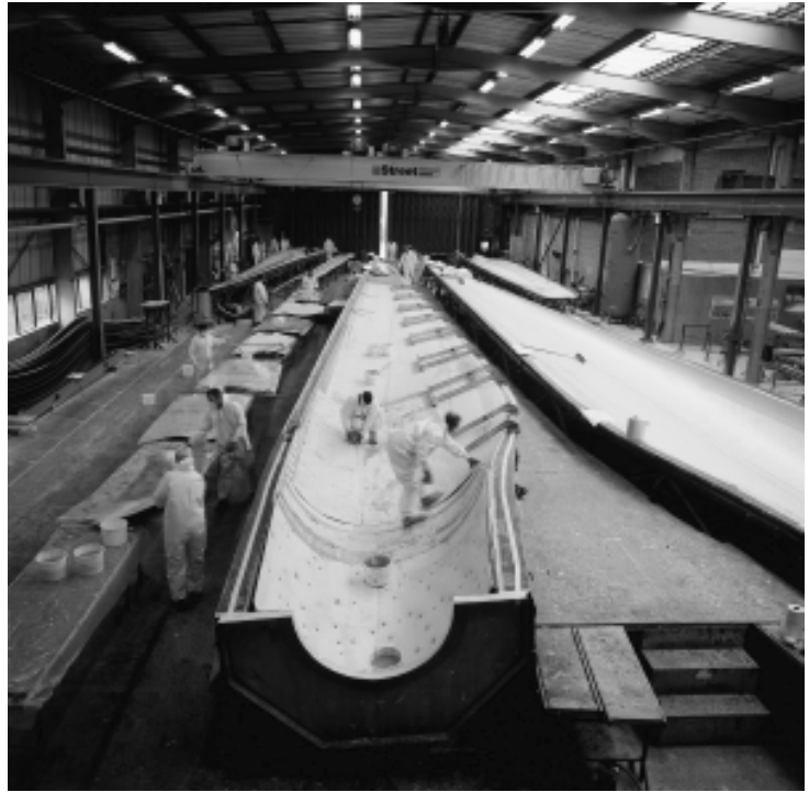
Workers assemble rotor blades. Photo courtesy of NEG Micon.
